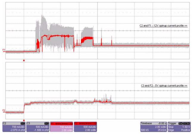
Figure 6. Typical ST3146756FC current profiles
