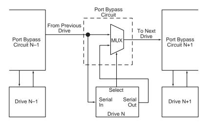
Figure 15. Port bypass circuit physical interconnect
