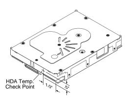
Figure 10. Locations of the HDA temperature check point
