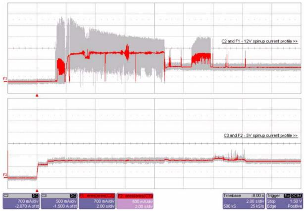
Figure 2. Typical ST3450056FC current profiles
