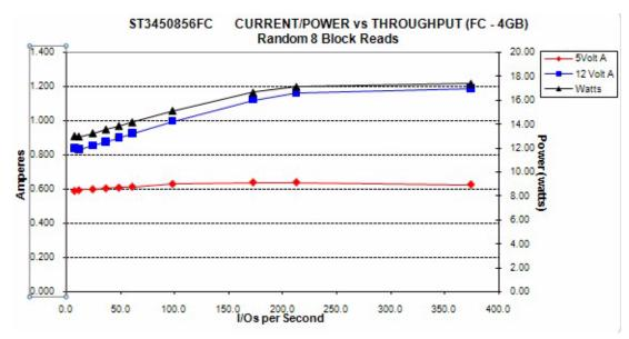
Figure 7. ST3450856FC DC current and power vs. input/output operations per second at 4 Gbit
