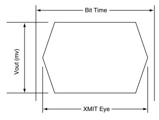
Figure 18. Transmit eye diagram
