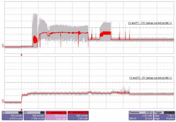
Figure 4. Typical ST3300056FC current profiles
