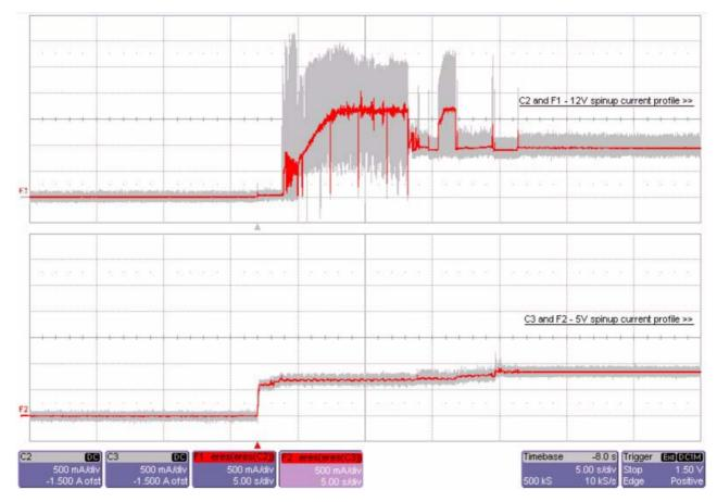
Figure 1. Typical ST3450856FC current profiles
