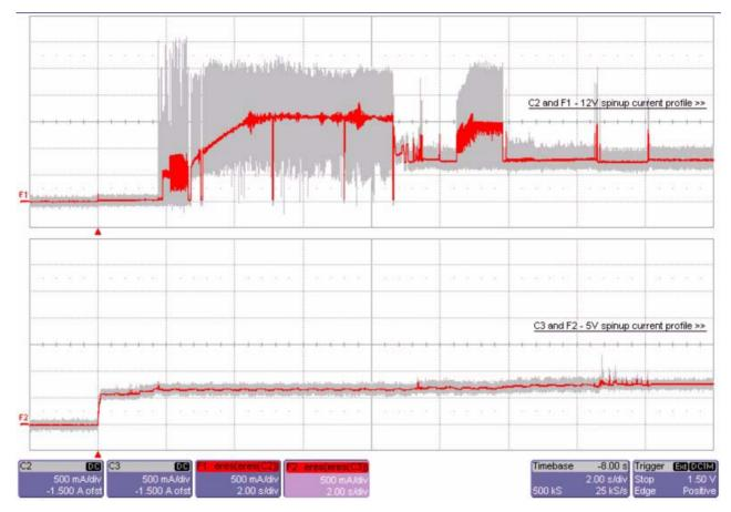
Figure 3. Typical ST3300656FC current profiles
