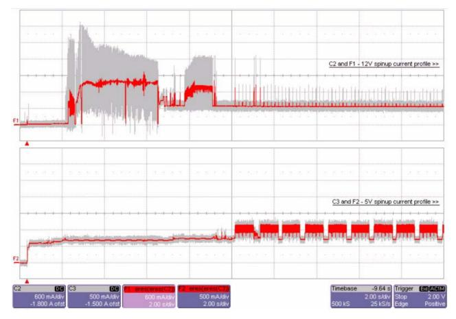
Figure 5. Typical ST3146356FC current profiles
